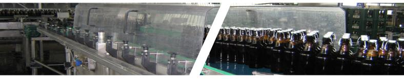
An inspection unit for the non-contact, reliable detection of leaks in glass bottles with metal crown caps, especially with a specific target internal pressure after the filling process, by evaluating vibration characteristics with state-of-the-art electronics and software algorithms.
